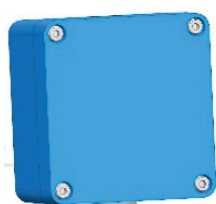
Large auxiliary aluminum terminal box for motor sizes 280–450. The size of terminal box ordered with these codes depends on the number of accessories ordered. 80 x 250 mm, max 30 strips. Earthing size M4.
